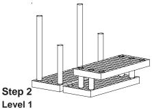
Position the Level 1 Panel on 12" legs overhanging outside edge as shown.
